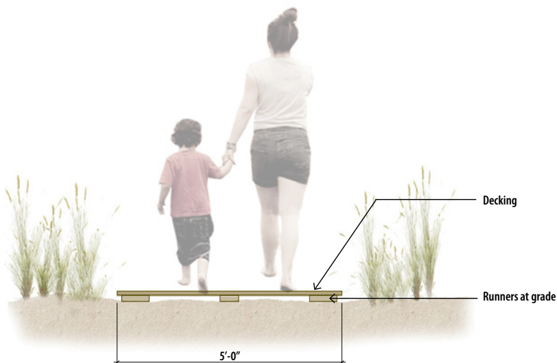
Figure 3 - Typical section of a Public Access Pathway.
